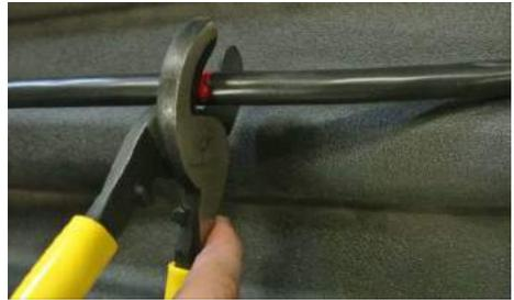
Step 6: Cut the jacketed portion off of the conductor about 8 inches.
