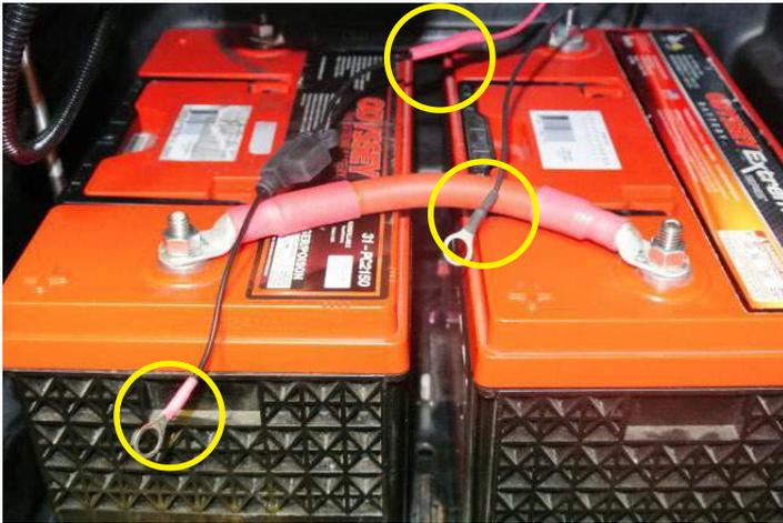
Step 10: Attached the 2 amp fuse holder to liftgate battery positive and the black ground wire to the liftgate battery negative.
