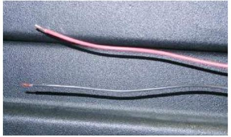
Step 9: Route the jacketed 2-conductor liftgate battery harness back into the liftgate battery box. Slide the supplied black ¼ inch heat shrink over the black wire. Slide (2) 2 inch pieces of the supplied red ¼ inch heat shrink over the red wire. Crimp on the 3/8 inch ring terminal onto the black wire. Crimp on the supplied 2 amp fuse holder to the red wire. Solder and heat shrink both connections.
