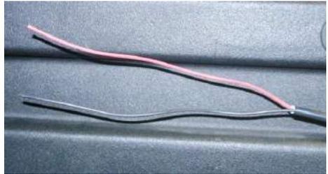
Step 7: Apply the supplied 3/8 inch black heat shrink where the jacket was stripped off.
