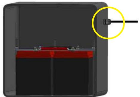
Note: Ensure that the 2-conductor jacketed wire enters the liftgate battery box through a dome nut or rubber grommet to prevent chaffing of wire, which could result in a possible electrical short in the system.
