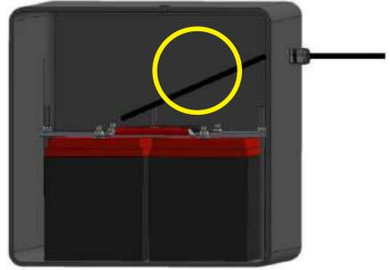
Note: If your battery box includes a slide-out tray, include enough slack to allow the tray to fully extend without tugging on the wire connections.
