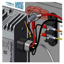
Step 5: Using a voltmeter, measure the voltage at the 2-pin terminal strip on the DC/DC converter charging plate:
