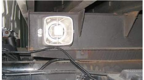
Step 3: Connect the buzzer ground to the truck battery ground and the positive to the main harness (quick connector).
