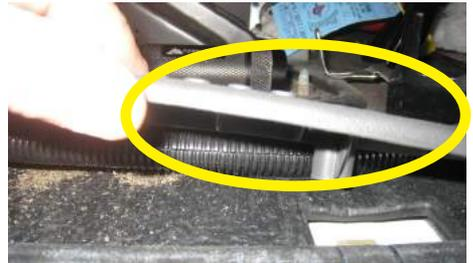
Step 2: Begin routing the harness under the seat belt, along the track where the door trim will be replaced back and through behind the kick panel of the truck.
