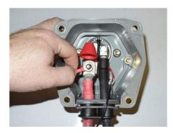
Note: Make sure the ring terminal of the smaller LED wire is on top of the larger dual pole cable.
