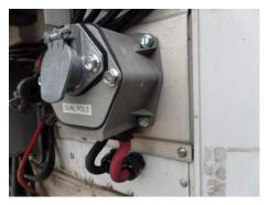
Important: To reduce the risk of electrical shock, make sure that the AC harness installation is complete before plugging in the dual pole cable from the vehicle into the trailer dual pole receptacle.
