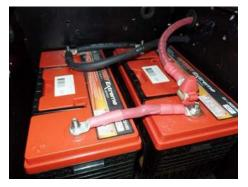
Important: Make sure that the AC harness installation is complete before making connections at the vehicle batteries.
