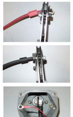
Step 6: Slide the 1/0 red positive cable through the black rubber grommet located at the bottom of the dual pole box. Place the 1/0 red cable over the fuse cube post and on top of the fuse cube. Place the smaller red LED wire on top of the 1/0 red cable. Secure this connection using the supplied fuse cube nut.
