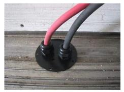
Step 3: Once the cables are through the trailer wall or floor, ensure they will reach the positive and negative posts on the vehicle batteries. Plan for a little slack in the cables, and cut off any excess cable.
