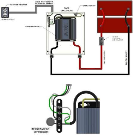
AC connections at the 4-terminal junction strip
