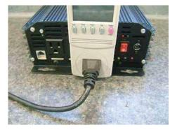
Step 4: The Watt/VA button is a toggle function button. Press the Watt/VA button once to display the Watt meter, then press button again to display VA meter. The LCD will display Watts as the active power, where VA is the apparent power (VA—Vrms Arms).
