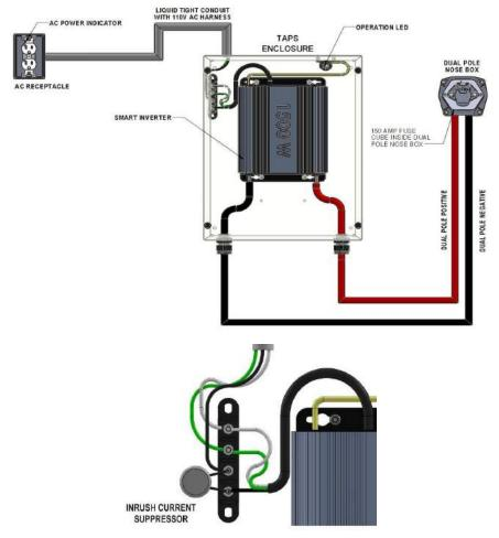
AC connections at the 4-terminal junction strip
