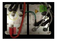
Note: On Carrier Vector reefers with two charging inverters, the reefer harness must be installed on the liftgate charging inverter and not the reefer battery inverter. Looking up from the bottom of the reefer unit, the liftgate charging inverter is the one on the left.
