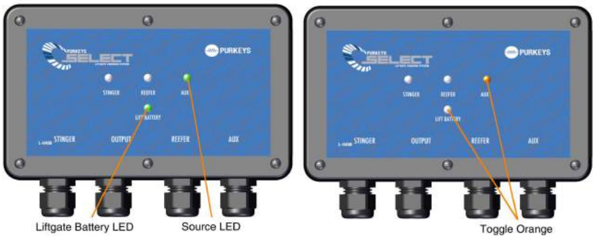
Figure 1: LEDs briefly turn green, toggle orange, then repeat
