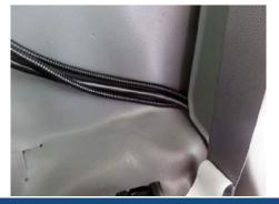
Step 9: Locate and remove the four door-step panel mounting screws. Carefully route the LVD wiring under the panel. Reinstall the panel and screws.
