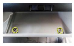
Step 4: Remove the center lower dash panel by locating and removing the lower mounting screw.
