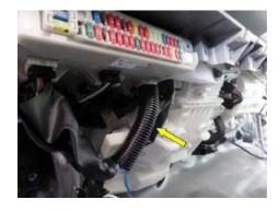
Step 15: Route the Ignition Harness (purple) toward the passenger side of the vehicle. Connect the 10-pin connector of the harness to an unused mating 10-pin connector in the vehicle located directly behind the glove compartment. Complete the installation by reinstalling all dash panels and fasteners and reconnecting the negative leads at the vehicle battery.
