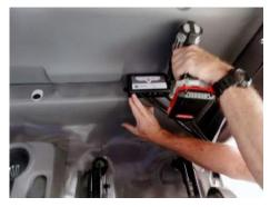
Step 8: Route all the LVD wiring behind the driver's seat belt cover.
