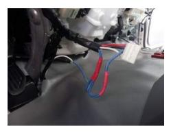
Step 14: Install the 3/4 inch protective conduit provided with the kit onto the spliced wiring.
