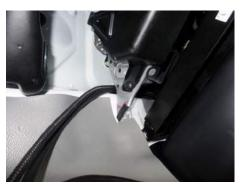
Step 12: Connect the Constant Power and Ground Harness ground (white wire) to a chassis ground. Be sure there is good metal to metal contact.
