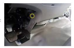
Step 6: Locate and remove the screw next to the fuse panel holding the mirror control panel in place. Carefully remove the rear view mirror control panel and the center lower dash panel.
