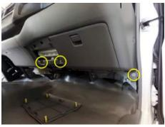
Step 3: Locate and remove the two mounting screws on top of the passenger side dash panel.
