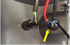
Step 11: Route the Constant Power and Ground Harness (blue and white wire) behind the steering column and toward the fuse panel. Avoid pinch points near steering column.
