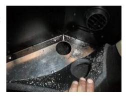
Step 5: The cable pass-through flange will be located next to the inverter. Use the supplied self-drilling screws and attach the pass-through.
