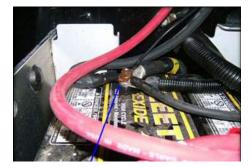
Step 13: Connect the inverter harness positive cable on top of the 100 amp fuse cube, install nut and tighten properly. Connect the factory cable on top of the 200 amp fuse cube, install nut, and tighten properly.
