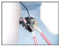
Step 7: Connect the inverter harness positive and negative cables respectively to the inverter. Also connect the 10 gauge chassis ground wire to the inverter chassis ground connection or inverter body.
