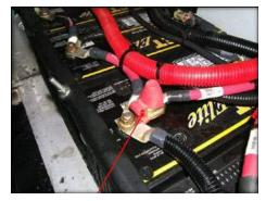
Step 11: Install the supplied dual fuse cube bracket and fuse cubes (the 100 amp supplied with the inverter harness and the 200 amp previously removed) back on the same battery post as the single bracket was removed from in the previous step. Do NOT connect the cables at this time.
