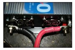
Step 8: Mount the inverter to the front of the bunk storage area. Push any excess cable back through the cable grips without putting too much strain on the cables. Securely tighten the cable grips.
