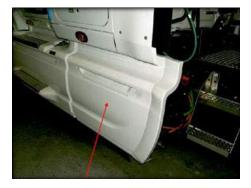
Step 2: A hole must be drilled in the floor behind the driver's seat for the inverter harness to be routed through. First pull the carpet back and make sure the wires that run under the carpet are out of the way and do not get damaged when drilling the hole. There is also a harness under the floor that can be damaged if the hole saw is ran past the floor when drilled.
