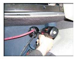
Step 6: With the cable grips loosened, slide enough cable through to be able to make the connections to the inverter. Tighten the cable grips to hold the cables in place.
