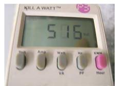
The KWH/Hour button is a toggle function button. Press the KWH/Hour button once to display the cumulative energy consumption since power was applied to the unit. Press the button again to display the cumulative time since power was applied to the unit.
