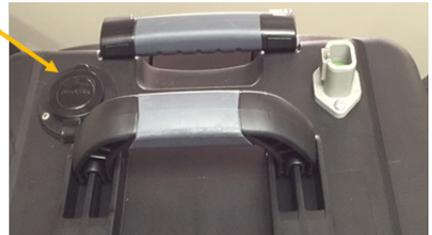
Step 5: Position the Direct/Select switch to system being demonstrated. Use the adjuster knob to raise or lower the liftgate battery voltage to simulate the following:
