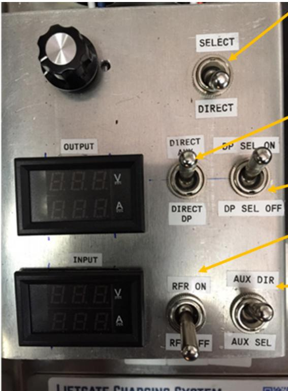
Determines which system gets liftgate battery connection
