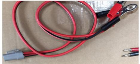
Step 2: Connect positive wire (red wire from 30 A CB) and negative wire from P1020 plate to an external battery. (Liftgate Battery)
