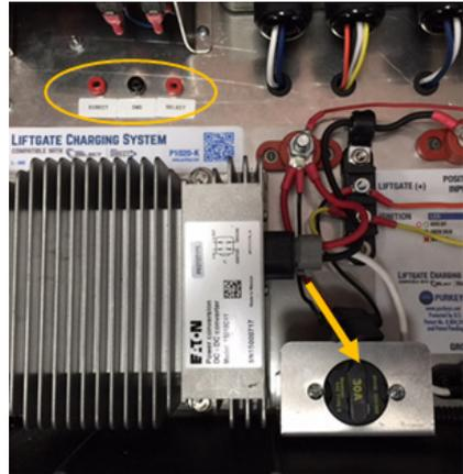
Step 4: Plug AC extension cord into the AC port located at the top of the demo box. This will be used to supply power to operate the internal power supply as adjust voltages for demonstration.
