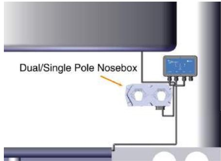
Note: Place the cable clamps along the reefer harness every 6 inches to ensure proper support for the cable. Avoid sharp edges and possible chaffing points.
