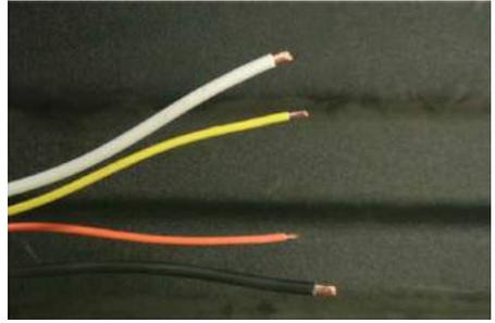
Step 9: Slide the supplied red 1/2 inch heat shrink over the orange, yellow, and black wires. Slide the supplied black 1/2 inch heat shrink over the white wire.
