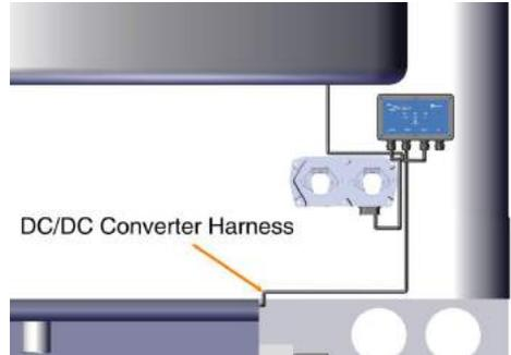
Step 2: Route the Select jacketed 4-conductor main harness in the center channel toward the back of the trailer. Secure with wire ties or cable clamps as you go.
