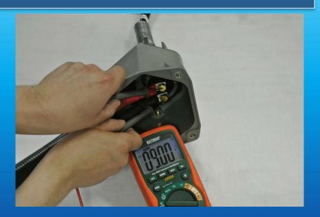
Green light on, but no voltage increase at liftgate batteries or any current flow
