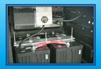
DC/DC charger that is powered from a dual pole cable from the tractor, controlled by an electronic "extender" module
