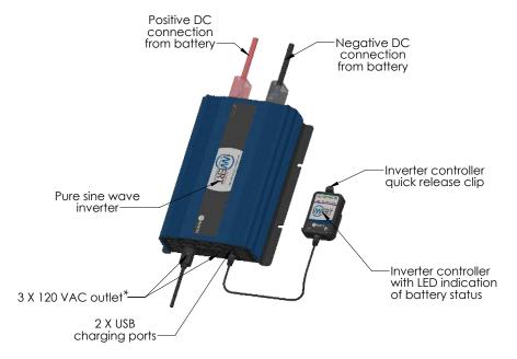
\*On the 2000 watt inverter, each AC outlet has a 15 amp circuit breaker/on-off switch. If the circuit breaker trips, reset the circuit breaker/switch by turning the switch off, then back on. The switches can also be used to individually switch the three AC outlets on or off.
