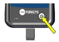
Step 3: To cycle to the correct setting, press the power button. Each time the button is clicked, a yellow light will indicate the setting.
