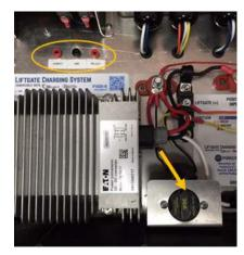
Step 4: Plug AC extension cord into the AC port located at the top of the demo box. This will be used to supply power to operate the internal power supply as adjust voltages for demonstration.
