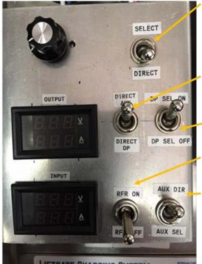
Determines which system gets liftgate battery connection
