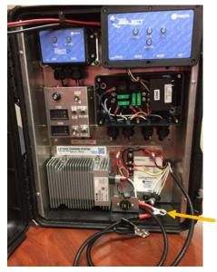
Step 3: Use the supplied leads with banana plugs and connect a multimeter to the receptacles inside the demo unit. Connect the black lead to Ground and the red lead to the positive of either the port marked Select or Direct.
