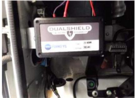
Step 12: Connect the ground wire from the LVD to a good chassis ground located near the LVD.
