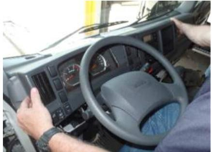
Step 3: Disconnect the hazard connector attached to the instrument cluster that was removed in step 2.
