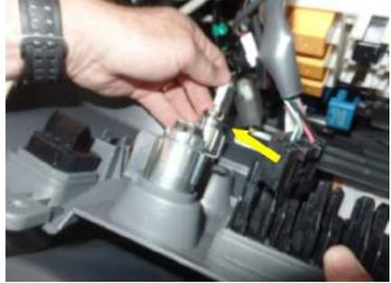
Step 10: Remove the extra connector from the holder and set the middle panel to the side.
