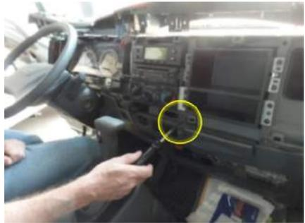
Step 7: Remove the plastic push rivet located on the lower left corner of the middle panel.
