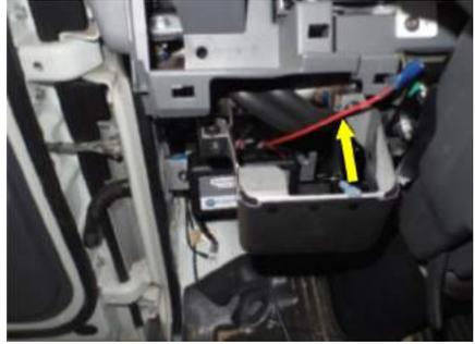
Step 18: Connect the LVD Output wire to the bottom terminal on the cargo light switch. The middle wire connects to the lights, and the top wire connects to a good chassis ground.
