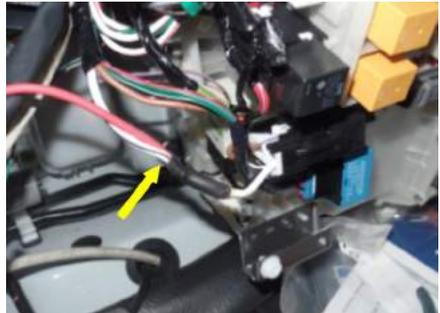
Step 15: Cut the red with yellow stripe cigarette lighter plug wire and connect the purple wire marked "Ignition" to the connector end of this wire. Heat shrink this connection.
