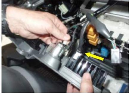
Step 11: Mount the LVD just inside the driver side door, using the supplied L bracket and hardware.
