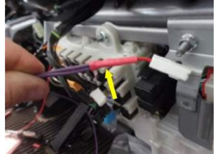
Step 16: Connect the other leg of the purple LVD ignition wire to the end of the red with yellow stripe cigarette lighter wire cut in step 15. Heat shrink this connection.
