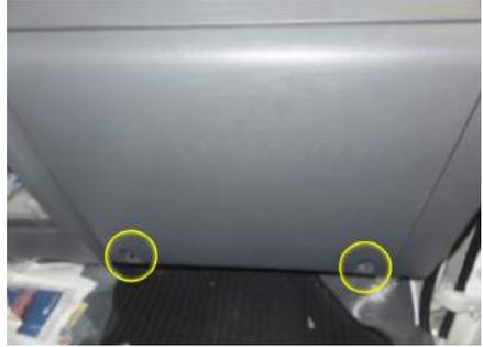
Step 6: Remove the 4 screws that secure the middle panel.
