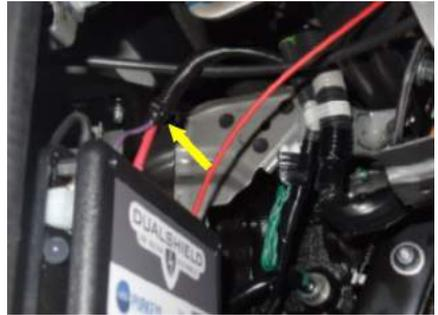
Step 14: Connect the red wire marked "Battery Positive" to the white with black stripe wire on the blower motor relay connector. Heat shrink this connection.
