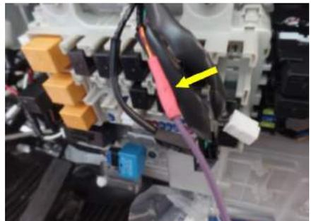
Step 17: Route the red wire marked “LVD Output” up toward the cargo box light switch.
