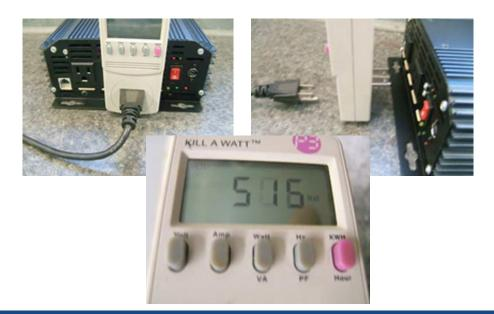
The KWH/Hour button is a toggle function button. Press the KWH/Hour button once to display the cumulative energy consumption since power was applied to the unit. Press the button again to display the cumulative time since power was applied to the unit.
