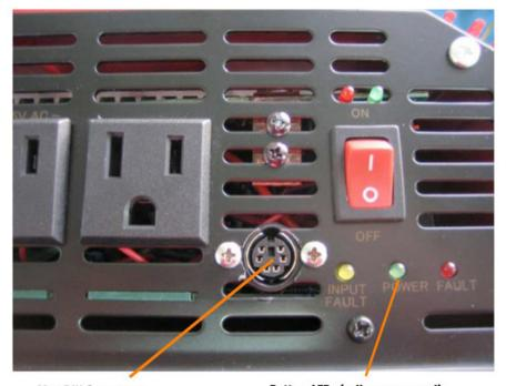
Mini DIN Connector: Programing the Inverter Bottom LEDs (yellow, green, red): Indicate Inverter Functions
