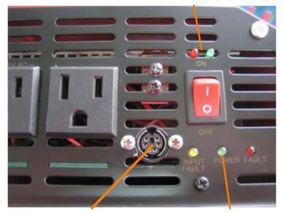
Mini DIN Connector: Programing and Timing Out the Inverter Bottom LEDs (yellow, green, red): Indicate Inverter Functions
