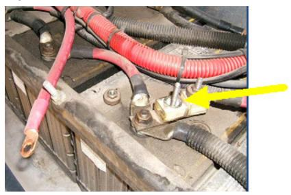
5. Short out the power inputs using a capacitor drain tool by connecting the positive and negative on the inverter. This will drain the internal inverter capacitors. See image below.
