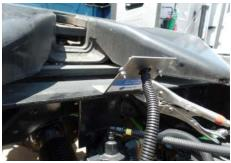
Step 6: Mark and drill a hole that will be used to secure the bracket to the cross member using a 5/16" drill bit. Use the supplied mounting hardware to secure the light bracket in place.
